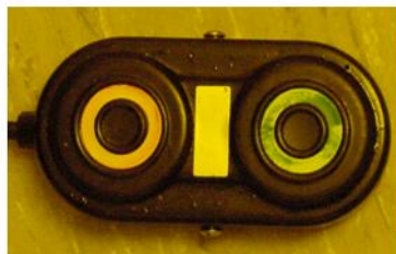
Foot Pedal Reset (red) and Start (green)
