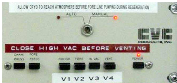
Fig. 1. Automatic Valve Control Panel
